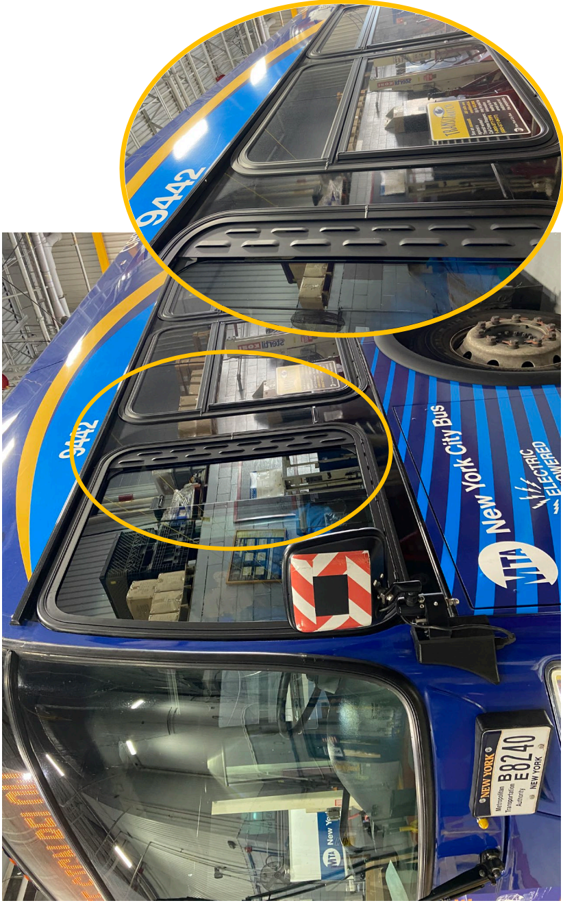
Fresh Air Vents Louvered-style operator window is being tested on 11 buses
